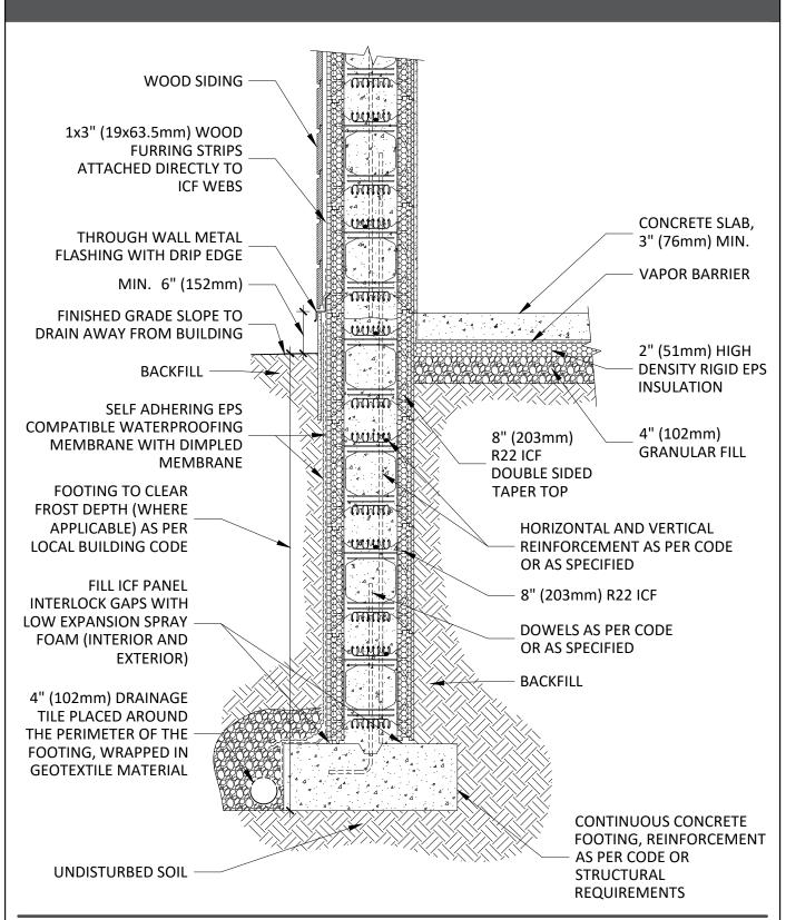
8" R22 ICF FROST WALL TO 8" R22 ICF WITH CONCRETE SLAB ON GRADE
