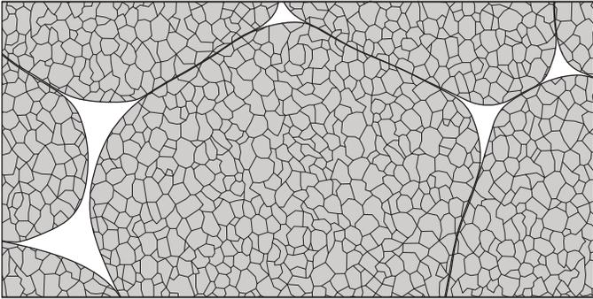
Expanded Polystyrene (EPS) foam cell structure (25x)
