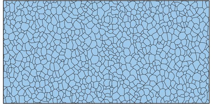
Extruded Polystyrene (XPS) foam cell structure (25x)
