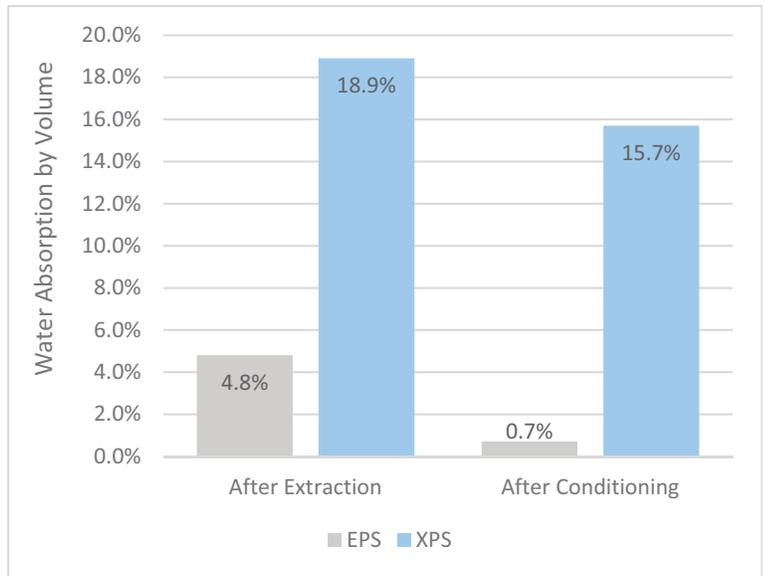
Stork Twin City laboratory water absorption testing results
