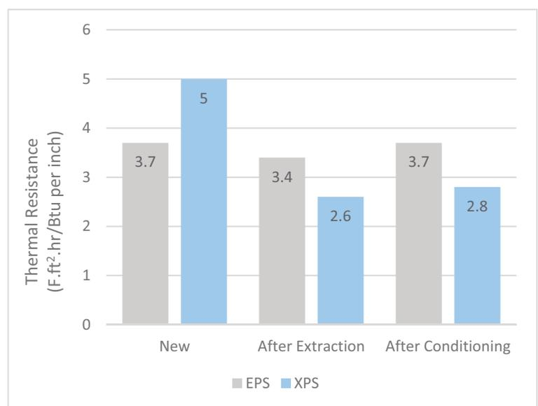
Stork Twin City laboratory thermal resistance testing results
