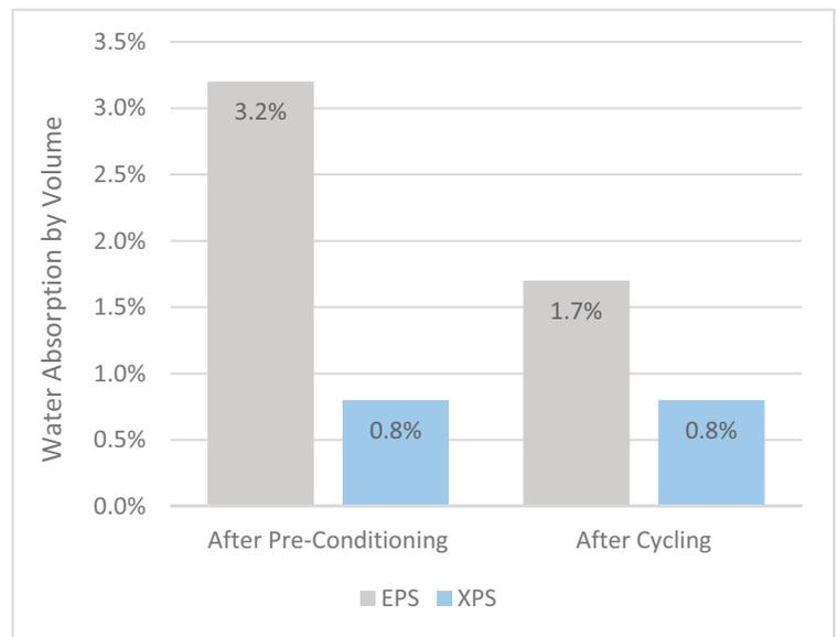
Intertek Testing Services laboratory water absorption testing results
